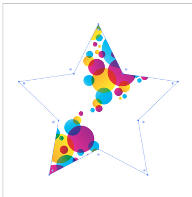
FIG 8.14: The star shape being used as a clipPath for the circles .
