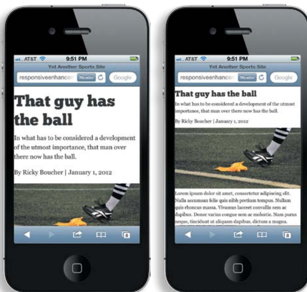
Figure 3.6 A 320px-wide device will display normally if the initial-scale is set to 1 (left). With the initial-scale set to .5 (right), the page will appear zoomed out.
