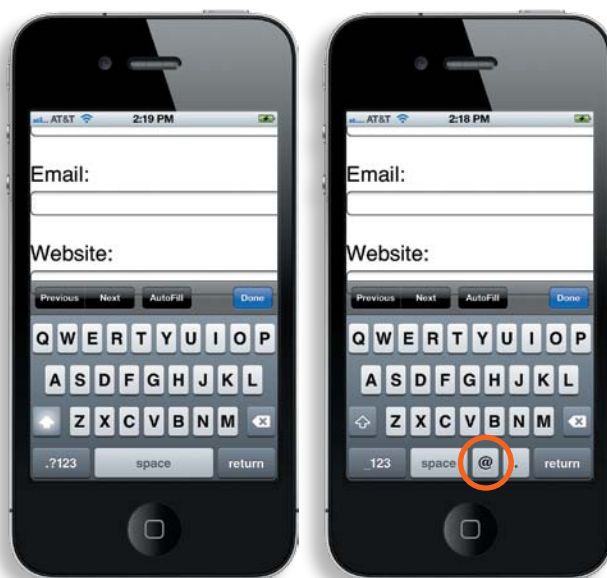
Figure 9.2 When iOS sees the “email” input type, it subtly adjusts the layout of the keyboard (right).
