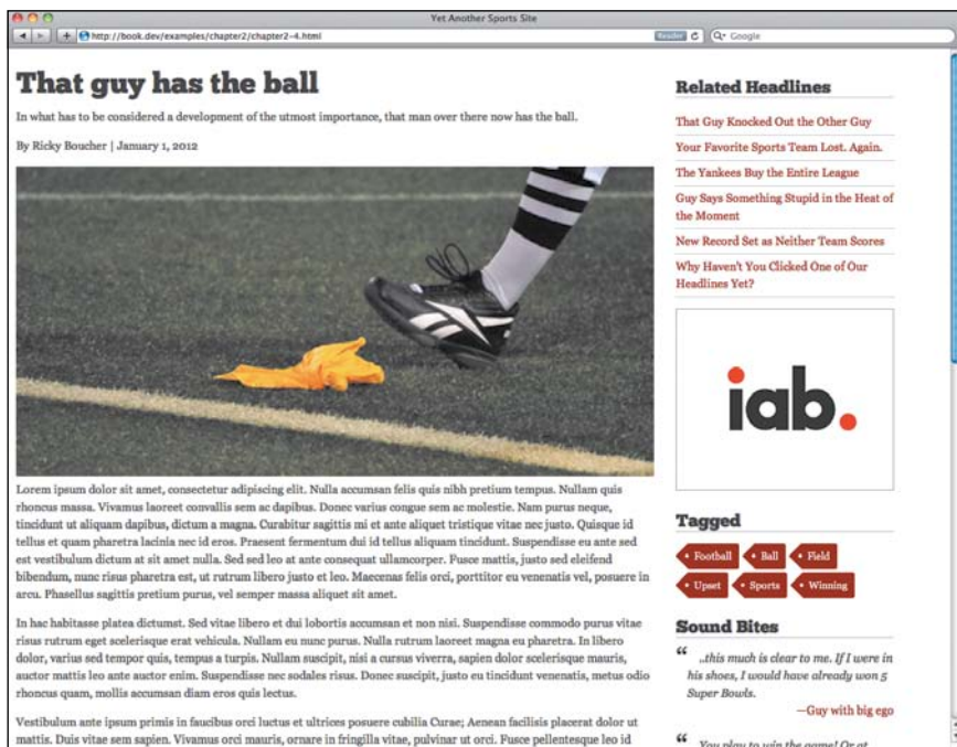
Figure 2.7 Using display:table-cell , the sidebar now stays a fixed 300px size while the main column adjusts to fill the remaining space.
