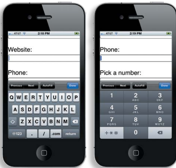
Figure 9.3 HTML5 input types, such as “url” (left) and “tel” (right) provide additional information to the device so that it can optimize the keyboard for users.
