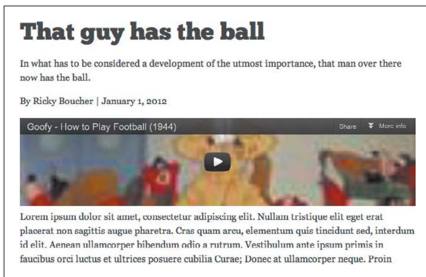
Figure 4.7 Unfortunately, using max-width: 100% and height: auto on video embeds will result in the video breaking the aspect ratio.
