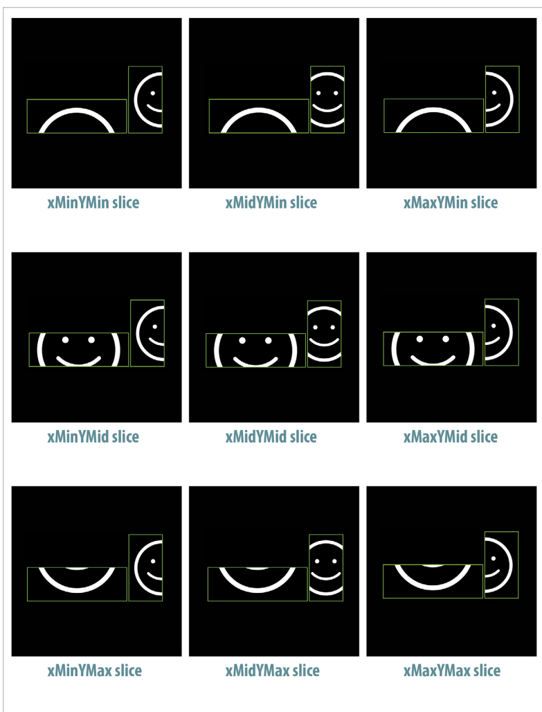
FIG 6.5: Examples of preserveAspectRatio values with slice .
