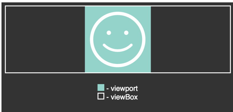
FIG 6.3: The viewport is enlarged, but no longer matches the aspect ratio of the viewBox . So by default, the image is drawn as large as possible without being cut off, and centered on the long dimension.
